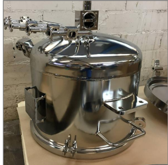
electropolished titanium container for the pharma
