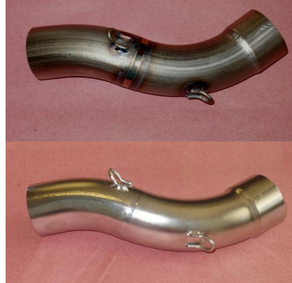
before and after electropolishing with POLIGRAT E 392
