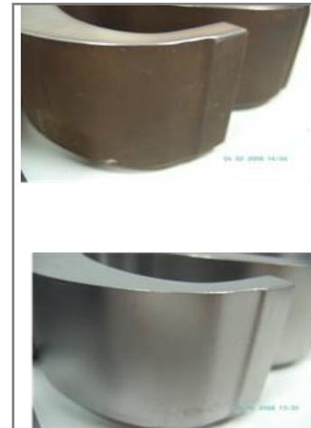
Surface before and after pickling with **POLINOX TB 100**, removal 70 µm
