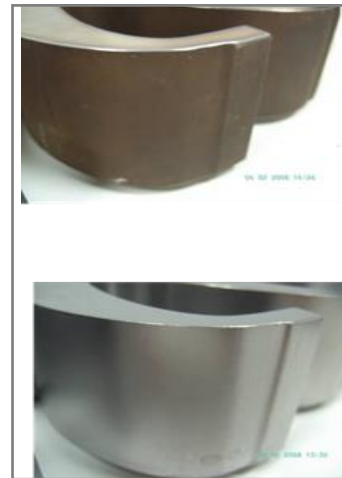
Surface before and after pickling with POLINOX TB 100 , removal 70 µm
