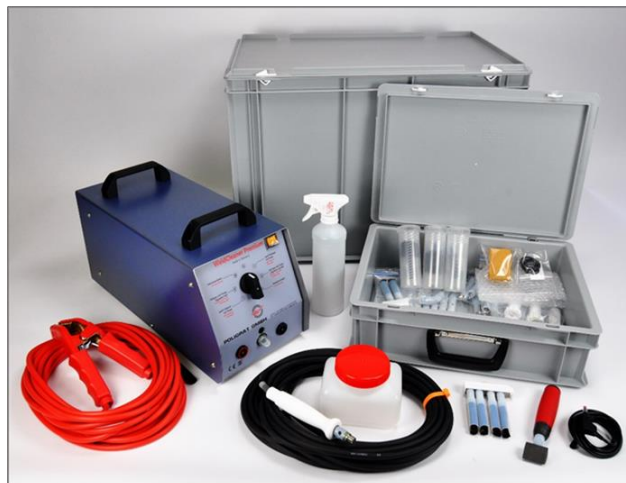
Weld scale cleaning with Carbon fibre brush
