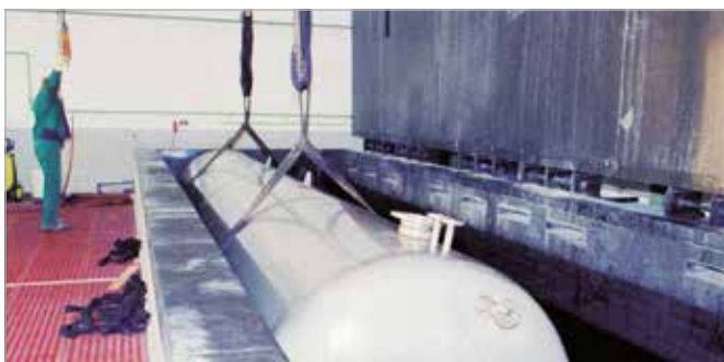
Immersion pickling in a 30,000 gallon pickling bath
